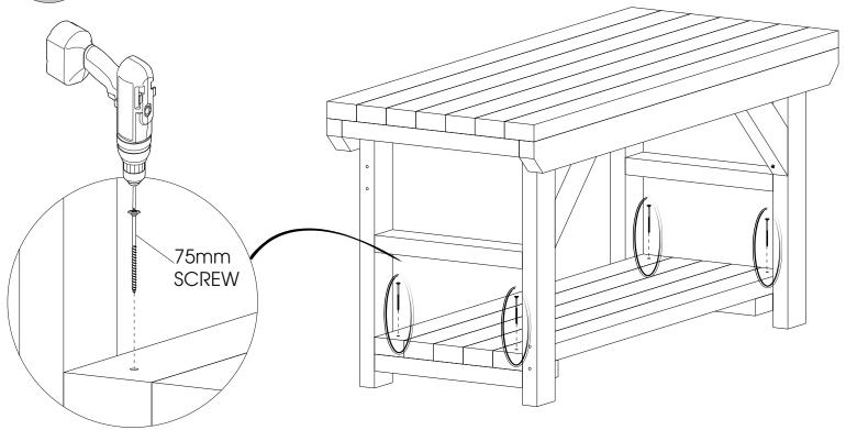
Attach the leg cross braces using 4 x 65mm screws on each leg
